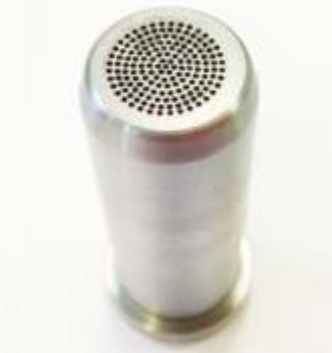
Drilling of holes in the filter - 163 holes \varnothing 0,45 \pm 0,05
