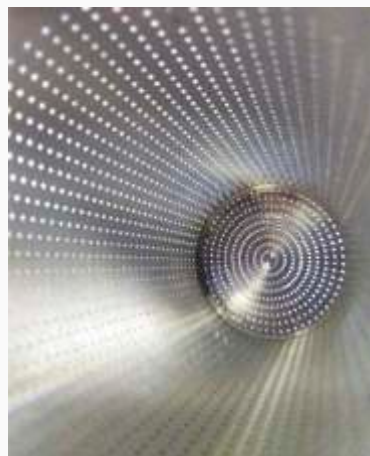
Drilling of holes in the cone type filter - 2301 holes \varnothing 0,3 \pm 0,03
